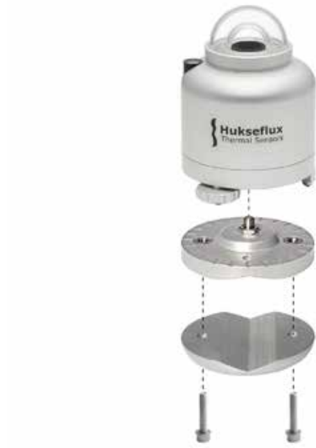
Figure 5.3.2.2 Optional tube levelling mount; installation requires a 4 mm hex key
