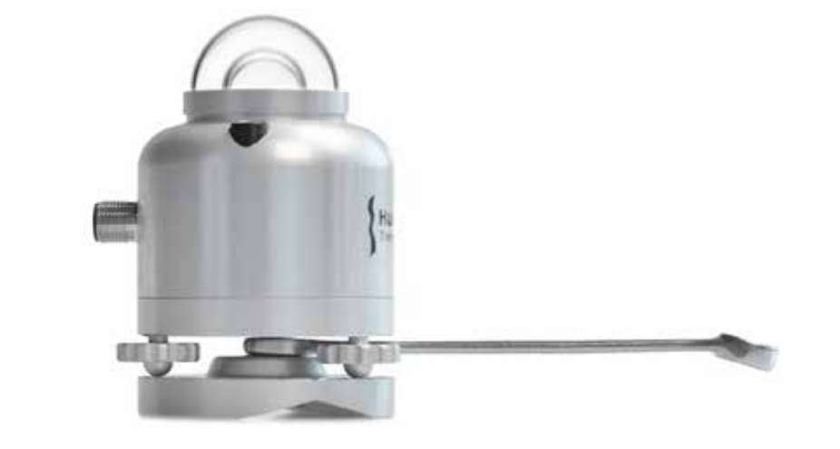
Figure 5.3.1.4 SR15 levelling mount seen from the side: (un)locking with a 10 mm spanner
