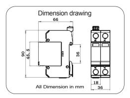
Type 2 surge arrester designed for low voltage DC system against surges at the boundaries from lightning protection zone OB-2and higher.
