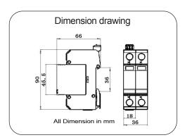
Type 2 SPD designed for low voltage system protection against surges at the boundaries from lightning protection zone 1-2 and higher.
