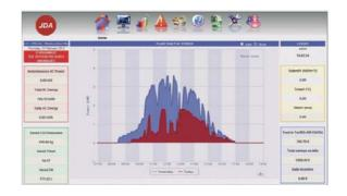
Yield index with an example of daily trend over the month. This information allows the PV plant owner to understand at a glance how the installation is performing versus the original engineering so to judge the investment payback time.
