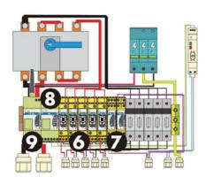
Master stringMoni® with switch disconnector, surge and fuses protection with measurements of V-A-kWkWh VIM-S, cell-air temperatures, irradiation, wind speed VIM-P and extended control features (VIM-O) and integrated master and web-server capability.
