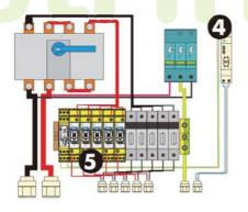
string Moni® with switch disconnector, surge and fuses protection with added measurement features.
