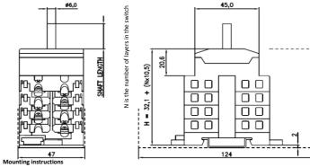
In the application all ratings have to be respected. When building the switch in an enclosure, the space envelope must be respected according to the applicable standards. After mounting, the wiring must be checked and the switch must operate smoothly.
