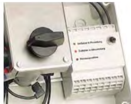
Electronic earth fault measurement
