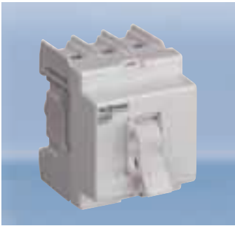
Off switch 3-pole 63 A 415 V~ Incoming circuit breaker for circuit distribution board, lockable in the "ON" or "OFF" position, maximum connection cross section 25 mm 2
