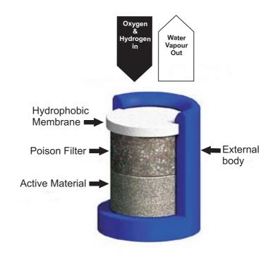
Today, SEC has extensive experience of the benefits of using Catalysts in our sealed VRLA cells, and we offer Catalyst equipped products in our 2 volt and 6-12 volt Monobloc batteries. We are also continuing our research and development program into new alternative Catalyst technologies and will be launching further new products in this area in future.
