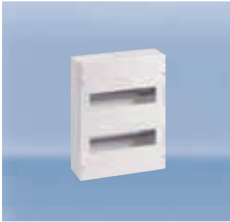
Surface mounted distribution boards 2 rows with N and PE terminals Dimensions: 275 x 346 x 74 mm
