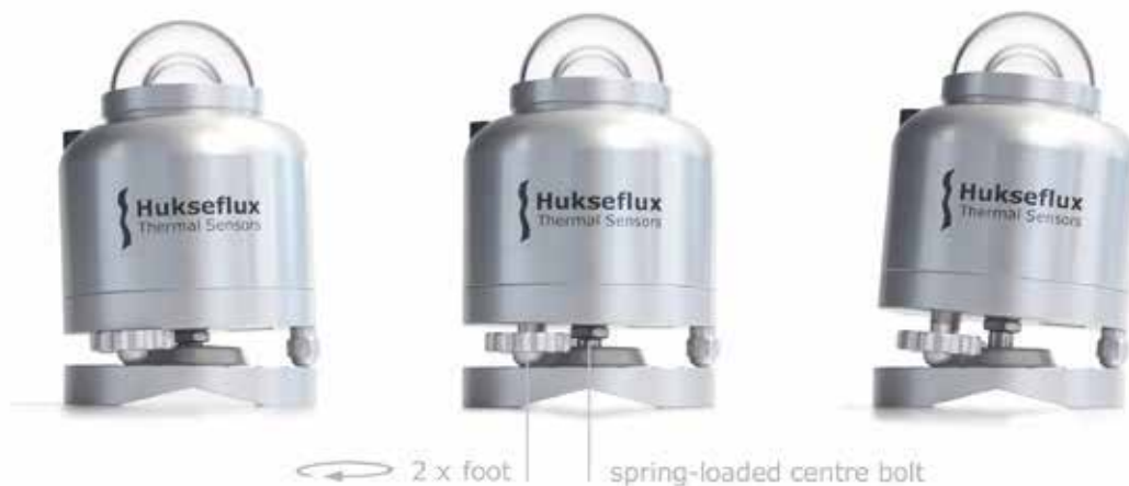
Figure 5.3.1.5 SR15-A1 locked on its optional levelling mount: by fastening (on the left) or loosening (on the right) SR15-A1's two adjustable feet, SR15-A1 can be levelled, judging by the bubble level. SR15-A1's static foot remains fixed. In all cases, ensure the legs of SR15-A1 fit into one of the small ledges of the levelling mount. Locking is in place, when the nut is turned all the way against the bottom plate of SR15-A1.
