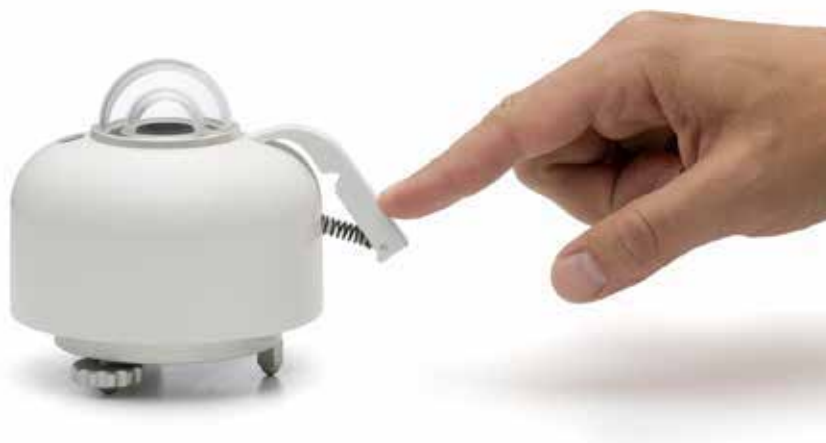
Figure 5.2.2 Installation of SR15-A1's sun screen
